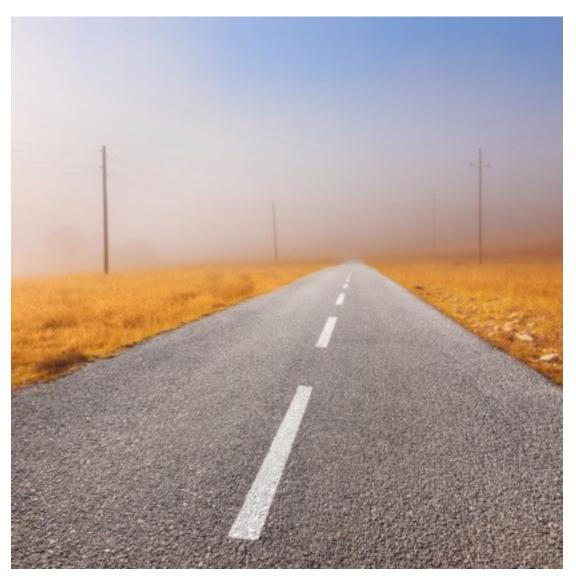
Most people believe that the dashed lines painted down the middle of a road are about 24 inches in length. And they're off by about 8 feet. US federal guidelines dictate that the dashed lines separating traffic lanes or indicating where passing is allowed run 10 feet in length. But a recent study showed that people grossly underestimate the length of those lines, and thus could be misjudging distances as they drive. That means they could be driving too fast.
